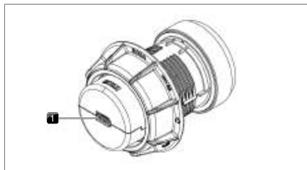
Fig. 4.69 Back of control knob with port
