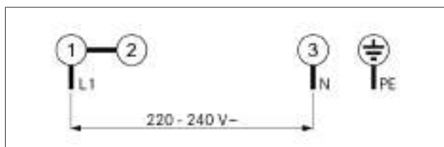
Fig. 4.87 1-phase connection diagram
