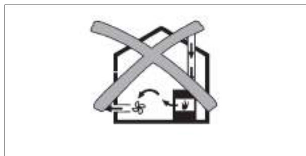
Fig. 4.1 Exhaust air installation – not permitted
